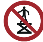
People are prohibited from going onto the platform
